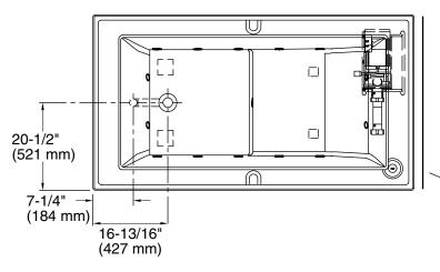
No change in measurements if connected with drain illustrated. (K-7193)
